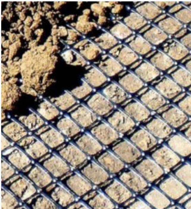
Figure 1:Grid Soil Reinforcement Source: (Sharma, Samanta, & Sarkar, 2019).
